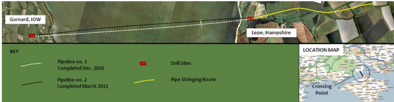
Aerial View of Drilled Crossing showing Drill Alignment & Pipe Stringing Site
